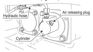
Figure 26. Removing Hydraulic Hose
